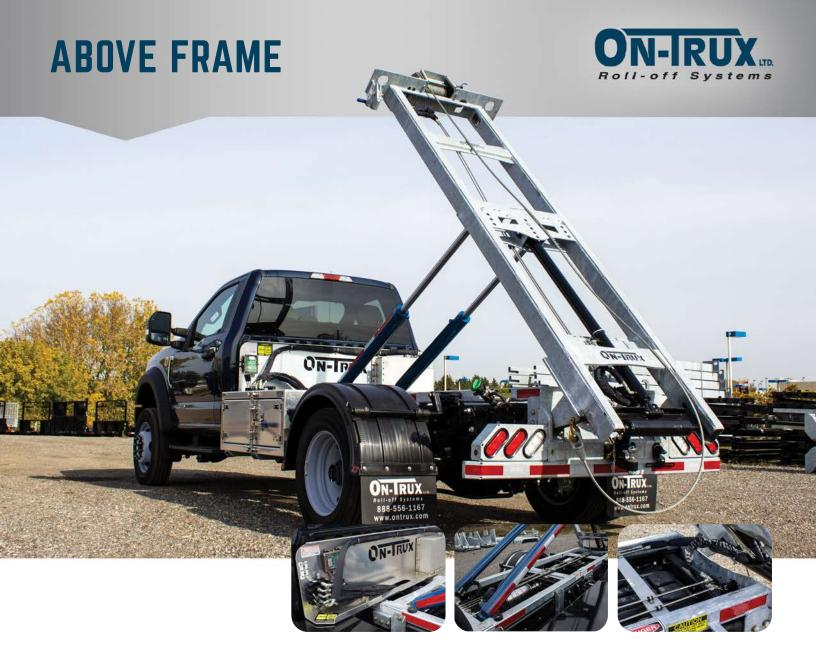
ON-TRUX Above Frame Roll-off Systems are designed for single axle trucks with 15,000 lbs. - 24,000 lbs. GVWR and can be installed on most new or used vehicles.
