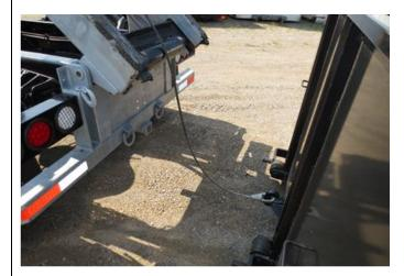
**16)** Safely exit the vehicle and remove cable from body and attach to holding hook. Leave slack in cable as shown below in both pics as this is the required amount to re-hook next body.
