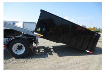
**15)** Depress <u>Hoist Up</u> until the stinger's roller almost touches the ground. This will allow the On-Trux body to rest gently on the ground. Depress (<u>Reeve)Cable Out</u> until the On-Trux body is rested on the ground. Engage the emergency brake so the truck may no longer roll.
