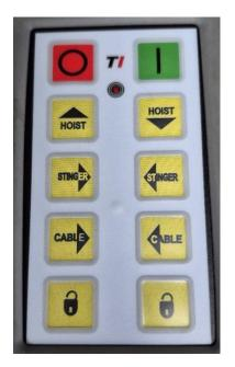
Buttons on the remote activate as you look at the side truck from the driver's side; the **Stinger Out** button is on the left and the **Stinger In** button is on the right. The **Cable Out** button is on the left and the **Cable In** button is on the left and the **Cable In** button is on the right.
