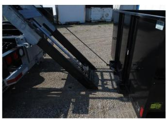
14) Apply brake, place transmission in neutral. Use brake to apply slight drag and depress (Reeve)Cable In, allowing truck to roll under the body. Use steering to correct any misalignment between chassis and body.
