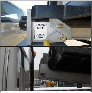
17) Depress <u>Stinger In</u> until the stinger is fully retracted. Depress <u>Hoist Down</u> until the ROS is docked on the frame of the truck. The rear section of the On-Trux body has been automatically locked by rolling over a locking mechanism. Turn off the clutch pump and disengage the PTO. (If you have a remote) Turn off remote by depressing red button. The LED on the remote will go out. For trucks with air ride suspension, always air back up after turning off the clutch pump/PTO.
