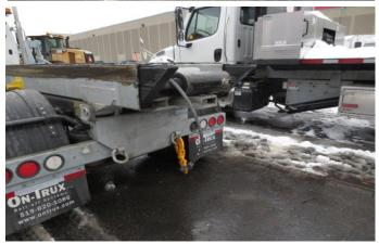
**17)** Re-engage PTO, Lower ROS (<u>Hoist Down</u>) until tightly against frame, <u>Shut off hydraulic pump (PTO)</u>. For trucks with air ride suspension, always air back up after turning off the clutch pump/PTO.
