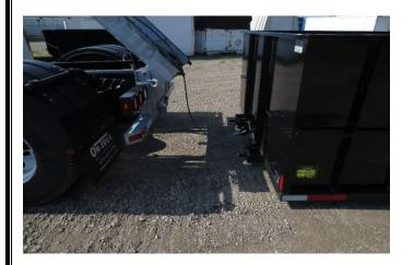
12) With cable attached drive the truck slowly forward gently until winch cable is tight & reengage PTO.
