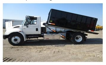
14) Depress (<u>Reeve)Cable Out</u> until the On-Trux body comes into contact with the ground. At this point, place the truck in neutral so the truck may roll forward as the bin is deployed. Depress (<u>Reeve)Cable Out</u> until the front of the On-Trux body is approximately 1 foot from the end of the main frame of the ROS.
