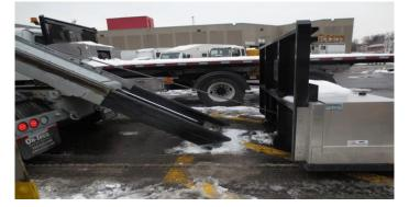
13) Depress <u>Stinger Out</u> until the stinger's roller almost touches the ground as shown in picture below. There should be no weight on the roller as the truck must roll on the ground surface.
